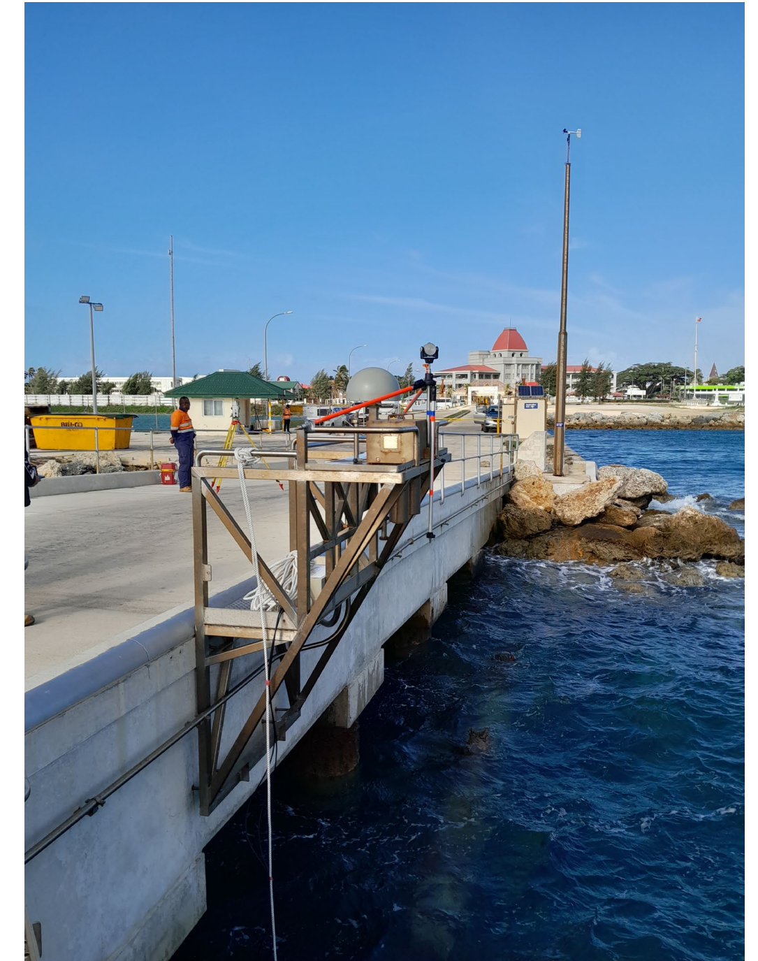
Radar Tide Gauge Station in Nuku'alofa, Tonga.
